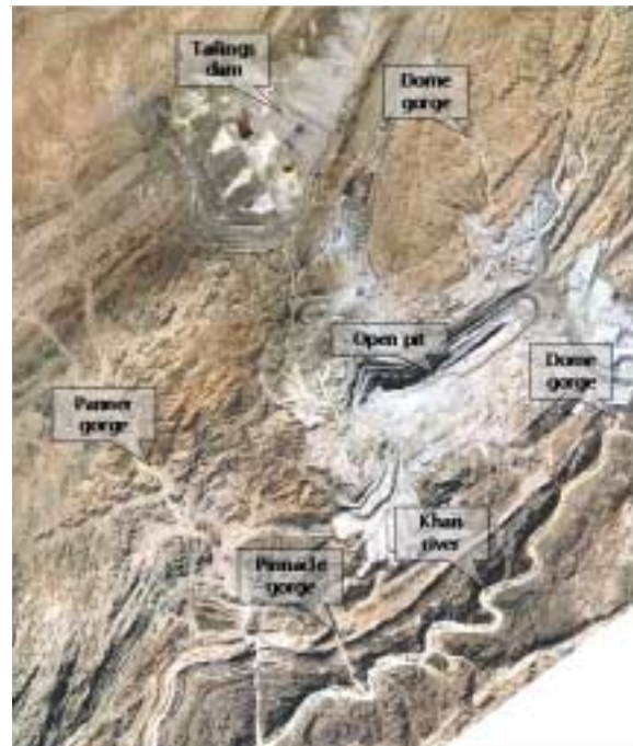
Figure 2. An aerial photo showing the tailings dam, open pit and processing plant of Rössing Mine
