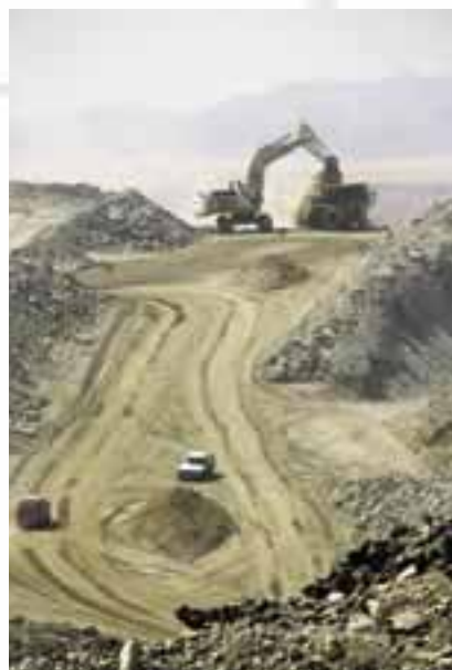
A shovel loads haul trucks with waste rock in the Pioneering area at Rössing where plants have been rescued prior to mining -- see page 33.
