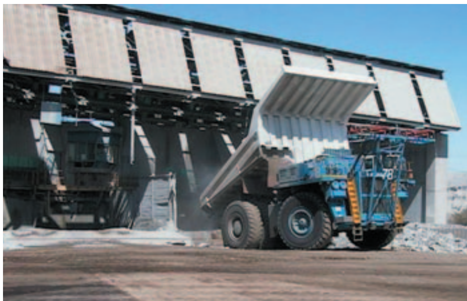
A 180 t capacity Haulpack truck dumping its load at the primary crusher. Photo courtesy of Rössing Uranium
