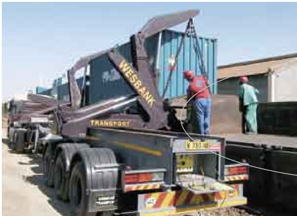
CONTAINER HANDLING: A container packed with drums of uranium oxide is loaded onto a railcar to transport the consignment to Walvis Bay harbour.
